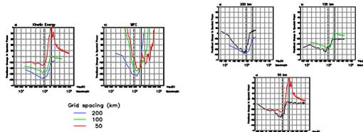
Figure 3: Fractional change in spectral power versus  $\log_{10}(k)$  and wavelength, small domain experiments for a) KE and b) MFC. The dashed line indicates  $k^*_{\text{max}}$  and the solid black line  $k^*_{\text{Nyquist}}$ .  $k$  in units of  $\text{m}^{-1}$ . Wavelength in units of m.
