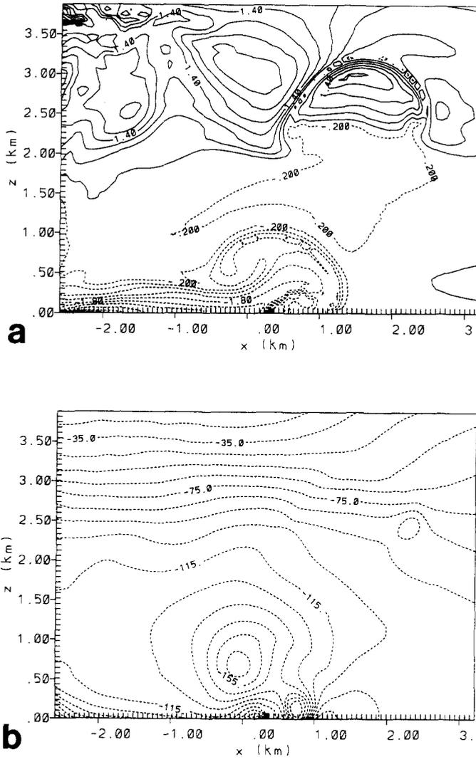
Figure 4: Fields at  $t = 5400$  s, for Grid 2: (a) Perturbation temperature. The contour interval is 0.4 k. (b) Perturbation pressure. The contour interval is 10 Pascals. (c) Horizontal velocity. The contour interval is  $1 \text{ m s}^{-1}$ .
