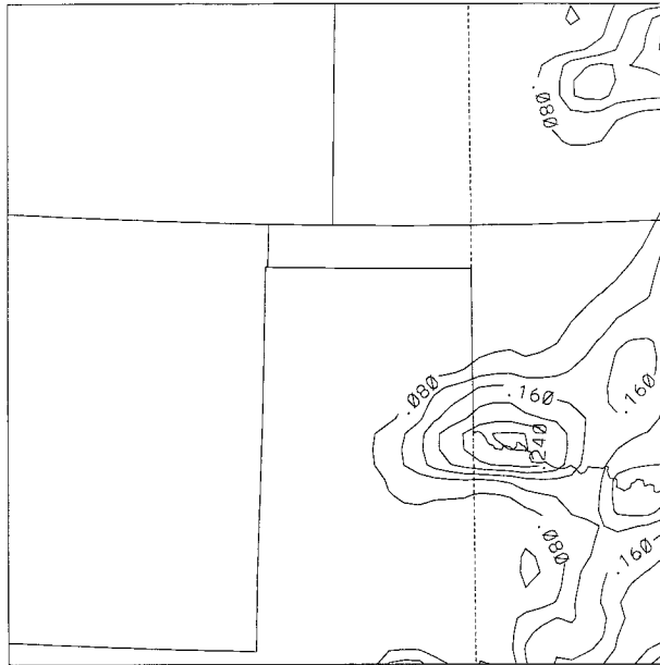
FIG. 4. Volumetric soil moisture distribution on grid 2 for the CONT simulation. Values represent fraction of total moisture capacity of the soil.
