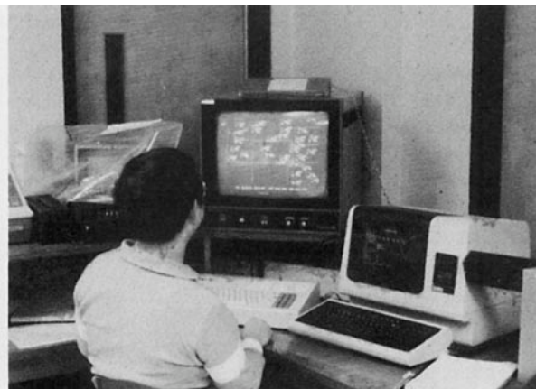
FIG. 4. The products of weather-lab software being displayed on the COMTAL Imaging System.
