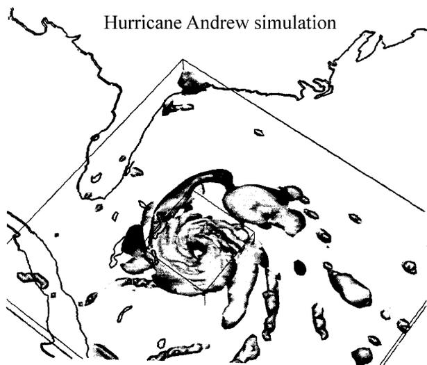
**Fig. 2.** Perspective view of hurricane Andrew from the southeast, shown at 66 hours simulation time. The shaded isosurface is condensate mixing ratio set to 1.9 g/kg. Only the 20 km and 5 km grids are shown, with the grid boundaries outlined. [From Eastman, 1995]
