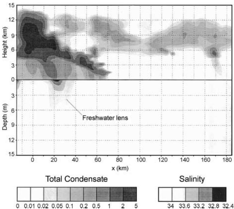
**Fig. 1.** A newly-formed freshwater lens and its parent storm at 19Z 22 December. The total condensate mixing ratio is shown in the upper panel (atmosphere) and the salinity field is depicted in the lower panel (ocean). The upper and lower panels have different vertical scales. [From Costa et al, 2001a]
