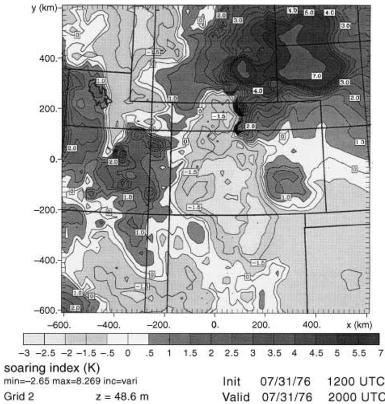
**Fig. 5.** Early afternoon forecast of the Cotton Soaring Index. Areas with values below  $-0.5$  K are conducive to thermals and are contoured with lighter shades. Areas with values above  $0.5$  K are stable and are contoured with darker shades
