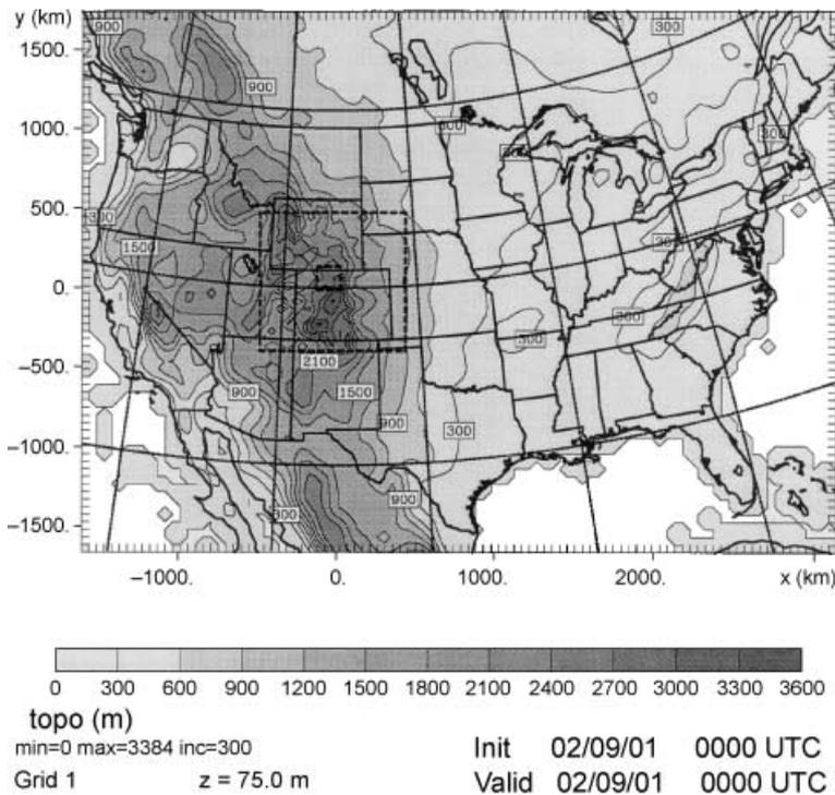
**Fig. 4.** Grid setup for realtime forecast version of RAMS. Entire Grid #1 domain is shown, with topography contoured. Nested Grids #2 and #3 domains are indicated as dashed boxes in the Colorado Rocky Mountain region
