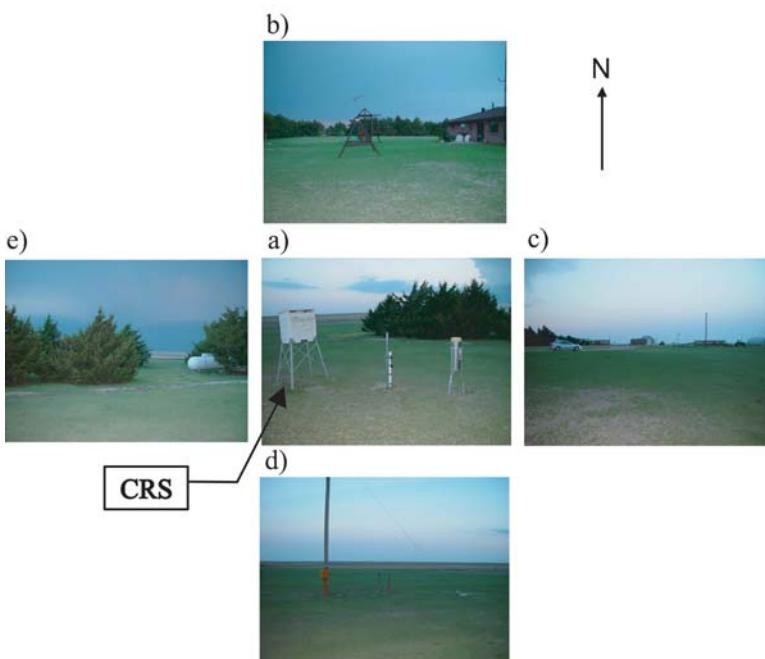
**Fig. 3. Photographs of the temperature sensor exposure characteristics of the COOP station Arapahoe 14N, near Arapahoe, CO. (a) The temperature sensor is a Cotton Region Shelter (CRS). (b)–(e) The exposures viewed from the temperature sensor looking north, east, south, and west, respectively.**
