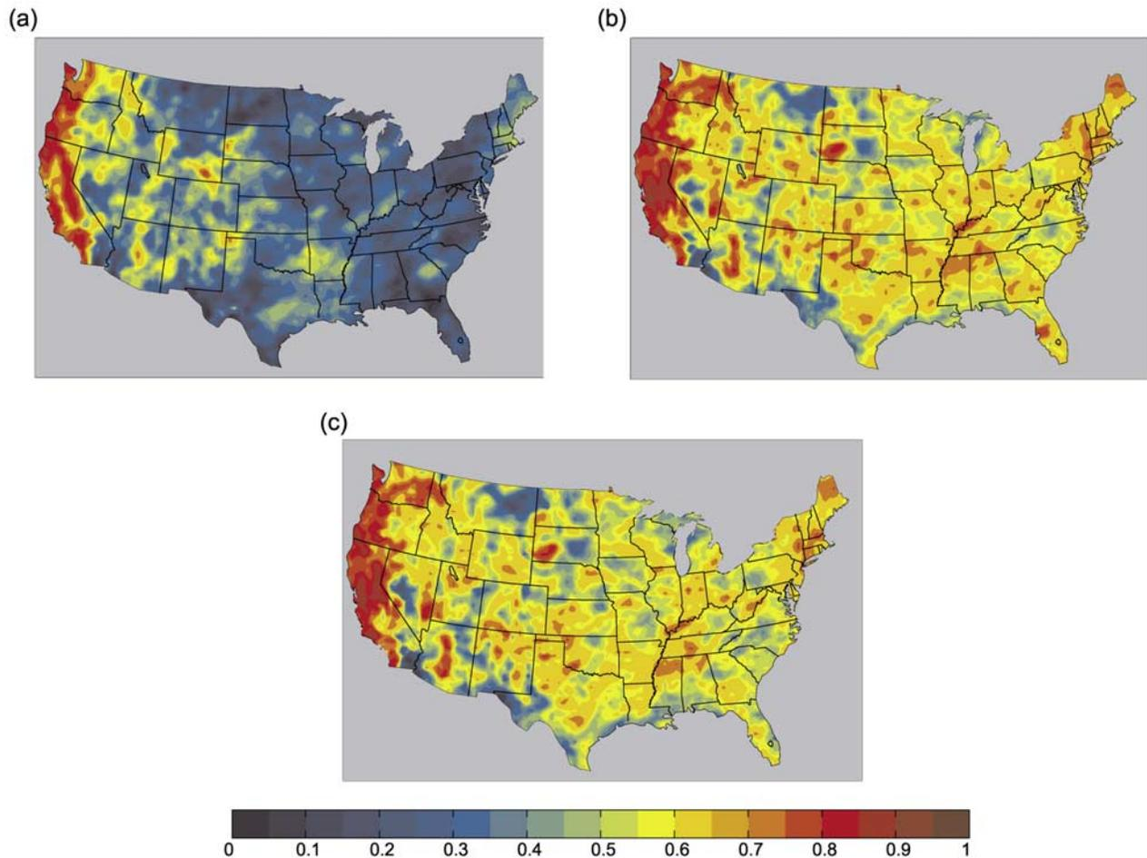
**Figure 8.** Correlation between time series of 24-h-accumulated precipitation simulations and observed values from NARR at every grid point for Jan–Dec 2000. (a) WRFS, (b) WRFS-FDDA-NOPBL, and (c) WRFS-FDDA-ALL.
