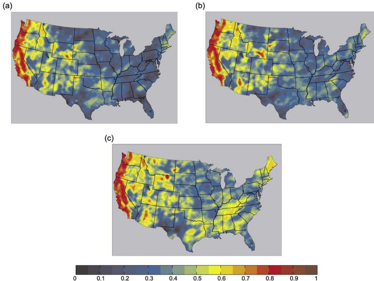
**Figure 4.** Correlation between time series of 24-h-accumulated precipitation simulations and observed values from NARR at every grid point during Jan–Dec 2000. (a) WRFS, (b) WRFM-30D, and (c) WRFM-7D.
