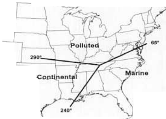
Fig. 1 Air mass classifications based on the air mass trajectory analysis. The polluted sector has high aerosol loading, marine region has cloudiness often associated with them and though the loading is less, the size of the aerosols is larger (possibly due to hygroscopic growth) and influences the DDR. The continental air mass has lowest aerosol loading and generally smallest DDR values. This is a generic representation and specific episodes may show significant variability (such as for the Mexico fire and aerosol plume in summer of 1998; which both the TOMS data and this study site showed a clear response for.
